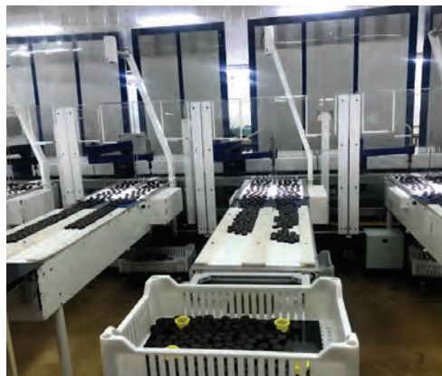
The packaging line is automated, featuring blue robot arms that can package 300 pieces in an hour. The company can even package different shapes by using a different hand for the various pieces, creating the assorted boxes of chocolates.
