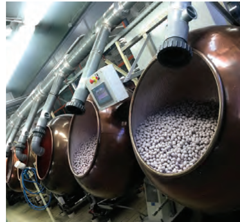
The main chocolate factory includes 10 marbling turbines for chocolate and sugar coating.
